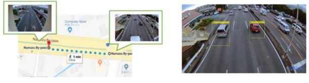
Vehicle detection system by CNN
