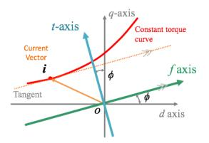
$\phi$  : Tangential angle of the constant torque curve Maximum Torque Control Reference Frame
