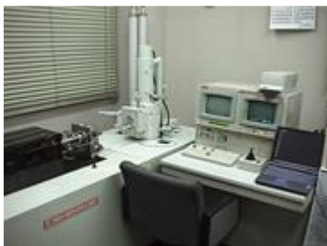
a) Fatigue test machine with SEM b) Fretting crack ( N_f = 7 \times 10^3 ) SEM in-situ observation of fretting crack behavior.
