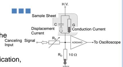
Fig.1 Detect Circuit
