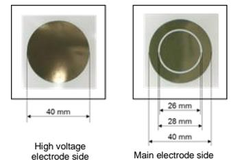
Fig. 2 Film's Geometry
