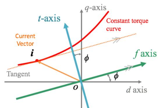
$\phi$  : Tangential angle of the constant torque curve
